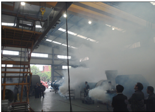
Fig. 14 Air curtain smoke blocking test by fog machine
