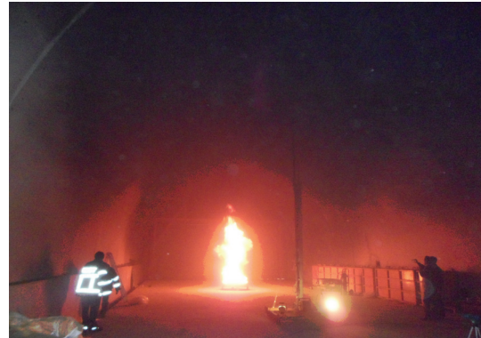
Fig. 17 Smoke blocking test of 2.5MW live tunnel fire (at KICT Hwasung fire research center)
