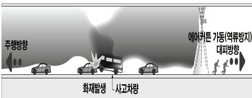
(b) Smoke spread prevention on tunnel fire
