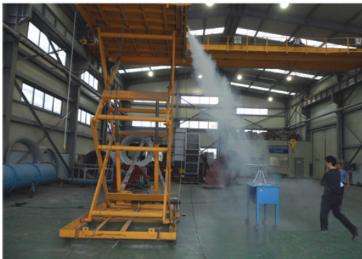
Fig. 15 Air curtain down stream air velocity check
