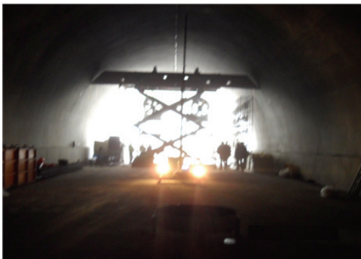
Fig. 16 Smoke blocking test case of 2.5MW live tunnel fire (at KICT Hwasung fire research center)
