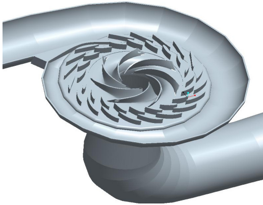
Fig. 1 Pump–turbine model cross section
