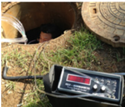
(c) micromanometer for pressure
