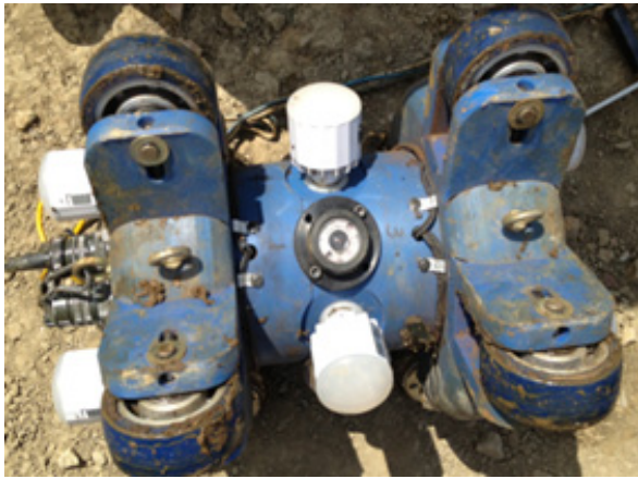
Fig. 4 Automatic robot having six cameras
