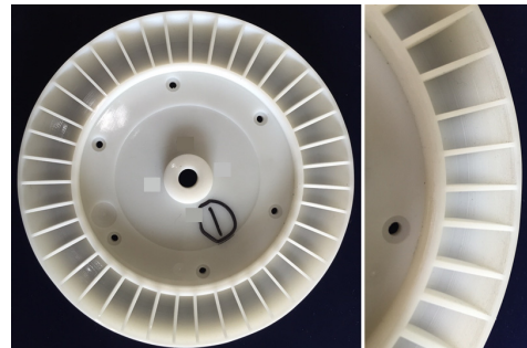
Fig. 3 Prototype of uneven pitch impeller by 3D printer
