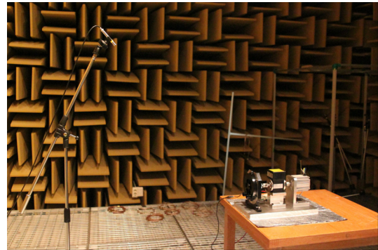
Fig. 5 Noise test in anechoic room
