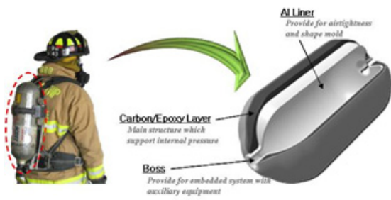
Fig. 1 Structural concept of Type3 cylinder
