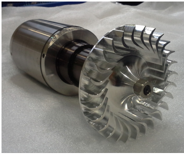
Fig. 1 Picture of turbine rotor connected with the generator rotor
