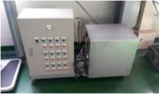
Fig. 9 Loadbank optimized for 30kW output power
