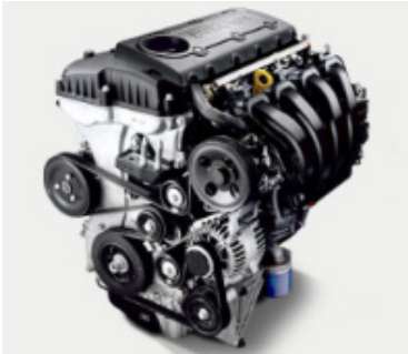
Fig. 2 Hyundai Theta II 2.4 L MPI engine
