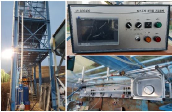
Fig. 4 Experimental apparatus of the horizontal branch pipe connected to a food waste disposer
