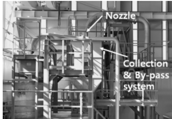
Fig. 9 Photograph of gravimetric calibration facility
