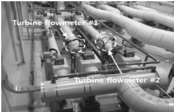
Fig. 8 Photograph of turbine flowmeter for flow test
