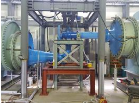
Fig. 1 Overview of test rig for Francis model turbine
