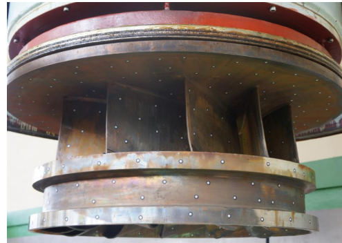
Fig. 3 Attached reference points for the scanning of the runner
