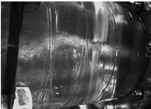
Fig. 18 Cavitation vortex rope visualization at Q_{11} = 0.19 and \sigma = 0.1
