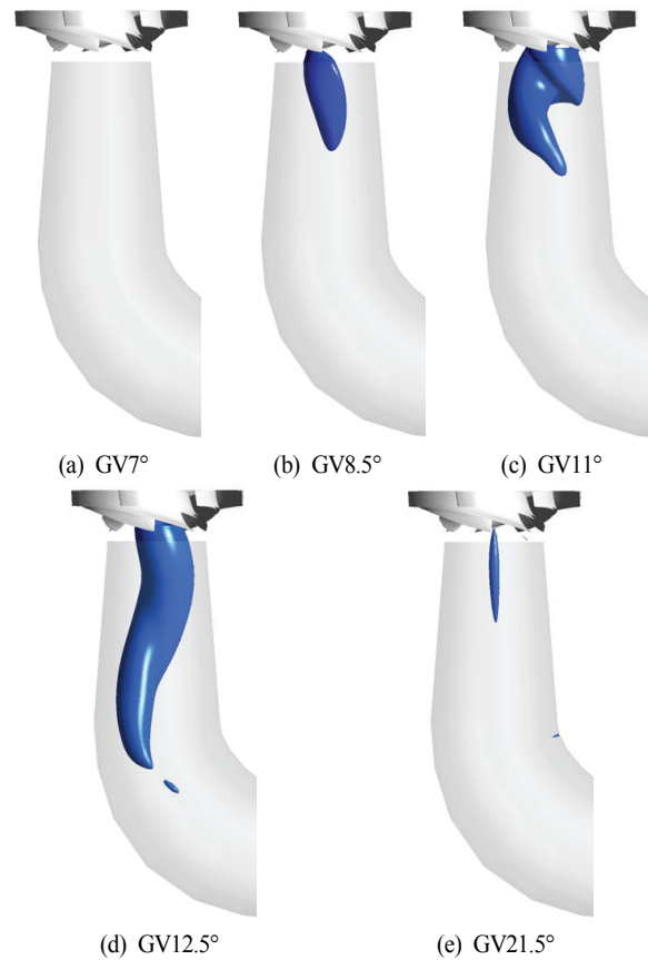
Fig. 7 Iso-surface distribution of time averaged pressure in the draft tube with various guide vane angles of a pump-turbine
