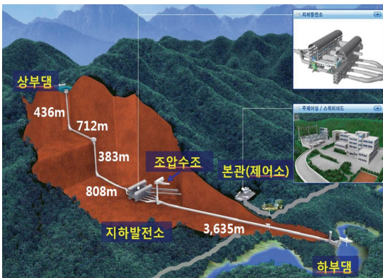
Fig. 2 View of pumped storage power plant
