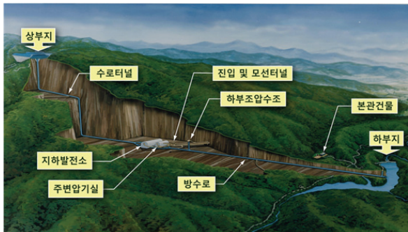
Fig. 1 Main facilities of pumped storage power plant
