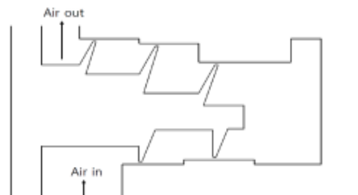
Fig. 5 Stepped solid double-sided labyrinth seals (6)
