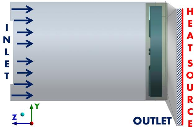
Fig. 2 Side view and boundaries of fluid domains
