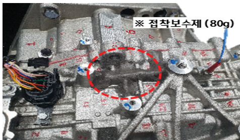
Fig. 6 Temporary Reinforcement of CASE
