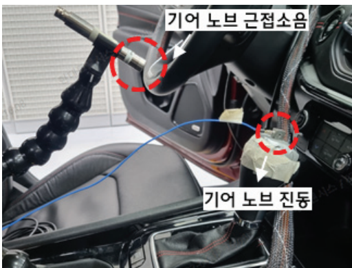
Fig. 15 Measurement Point of vibration and noise for shift knob
