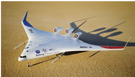
Fig. 2 NASA X-48B UAV with micro gas turbines (3)
