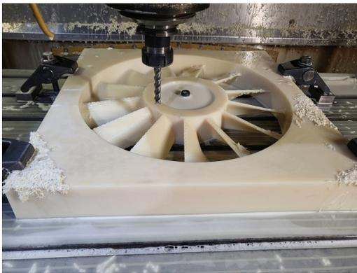
Fig. 8 Fan in fabrication process
