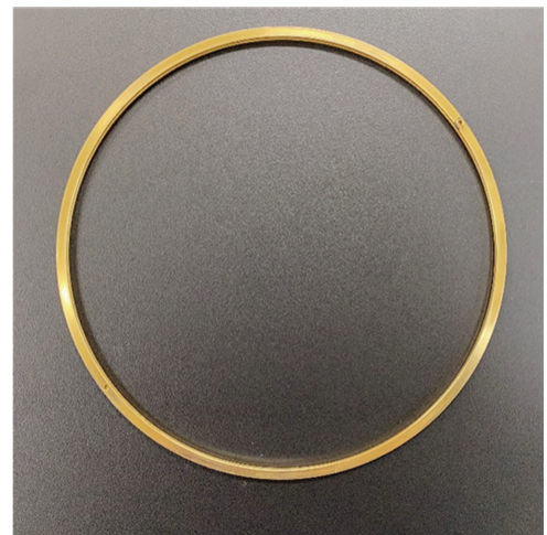
Fig. 3 (a) Schematic of main rotating part and seal components in cryogenic ball bearing test rig (b) brass ring
