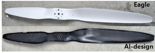
Fig. 15 Photo of fabricated propellers (top: Eagle-biomimetic, Bottom: AI-design)
