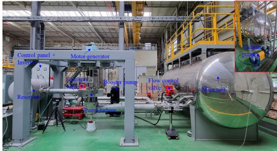
(b) Configuration of Lab-scale pump-turbine model
