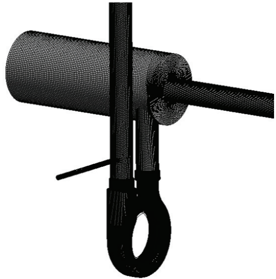
Fig. 5 Numerical grids of regenerative pump and ultrafine bubble generator
