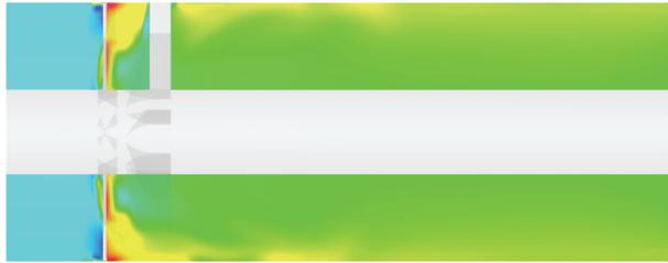
Fig. 11 Total pressure distribution of optimal fan impeller and outlet guide vane
