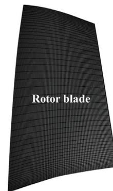
Fig. 7 Grid systems for numerical analysis of static structure
