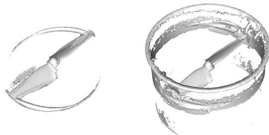
Fig. 8 Comparison of Vorticity Magnitude Iso-Surfaces between Ducted propeller and Unducted one
