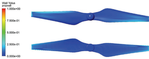
Fig. 4 Y+ distribution on the propeller wall
