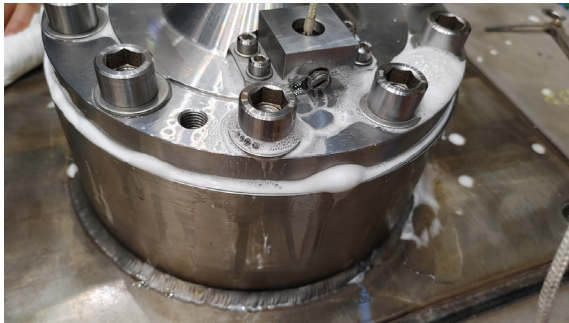
Fig. 14 Leakage test result of pneumatic system
