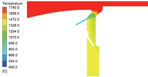
Fig. 12 Cross-sectional temperature distribution in the sealing region with injection angle at 30°
