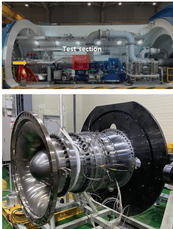
Fig. 4 Low pressure axial turbine and test facility
