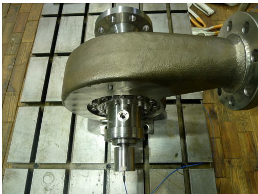
Fig. 14 Impact testing of turbine rotor
