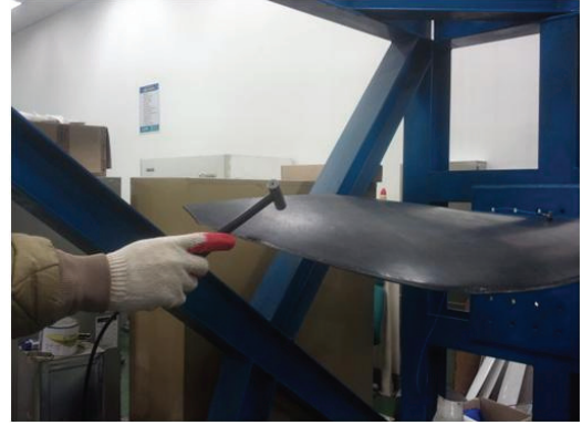
Fig. 19 Natural Frequency Test
