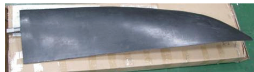
Fig. 16 Manufactured Composite Blade
