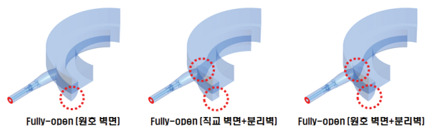
Fig. 4 3D modeling of sintering cooler flow field by air duct wall shape condition
