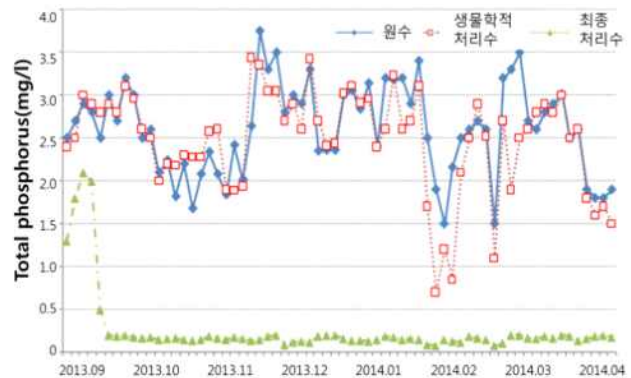
Fig. 6 Concentration(mg/L) of TP in the treated effluents by this wastewater treatment system
