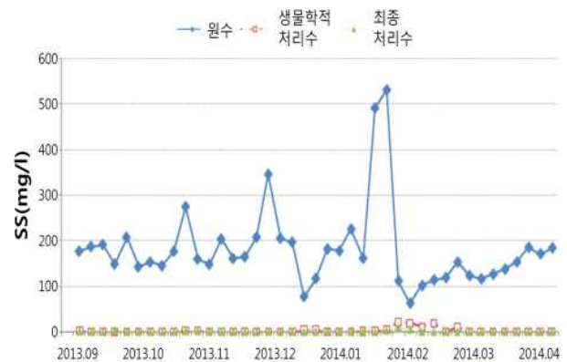
Fig. 4 Concentration(mg/L) of SS in the treated effluents by this wastewater treatment system
