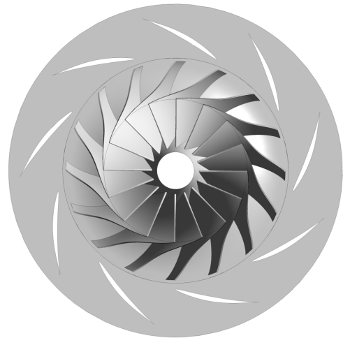
Fig. 2 Three dimensional view of the impeller and vane diffuser
