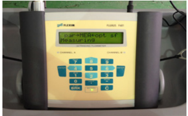
Fig. 2 Building place installed ultrasonic flowmeter
