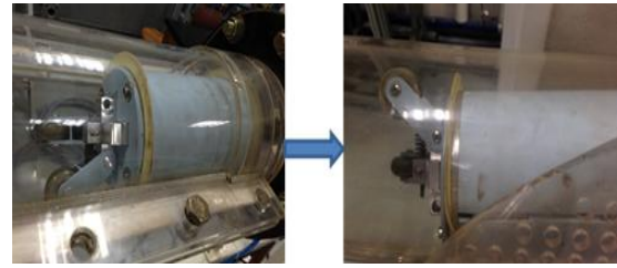
Fig. 12 Rotation of the capsule during the movement in the test facility
