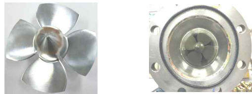
Fig. 3 The existing old runner model (left) of the propeller turbine installed in the inline pipe (right)
