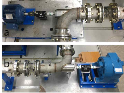
Fig. 2 The axial pump model(a) and (b)propeller turbine model
