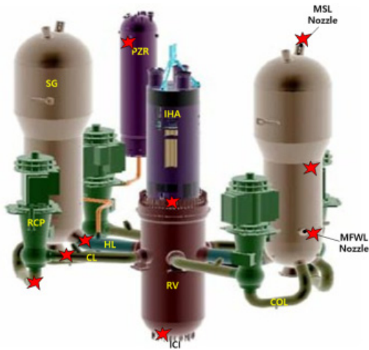
Fig. 1 Expected leakage points in reactor coolant system
