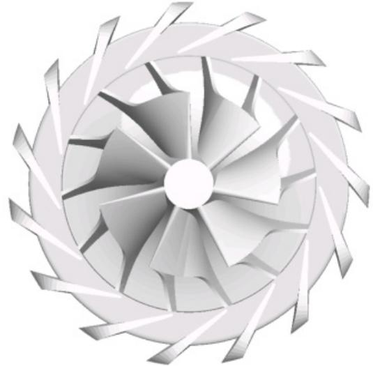
Fig. 1 3D modeled view of Jetcat RX300 engine compressor
