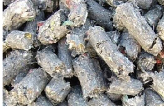
Fig. 2 Regenerated fuel pellets made from domestic waste
