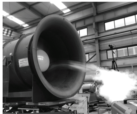
Fig. 2 Axial flow fan noise measurement
