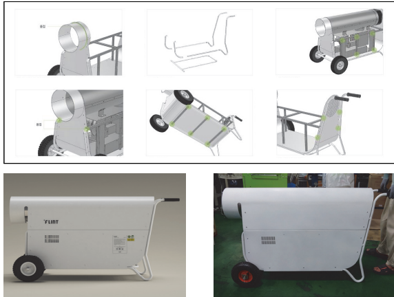
Fig. 13 Final design and production of prototype bio-agricultural hot air blower
