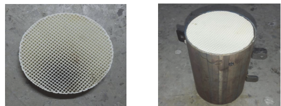
Fig. 4 Honeycomb Ceramic filter(left) and combustion chamber by filter (right)
