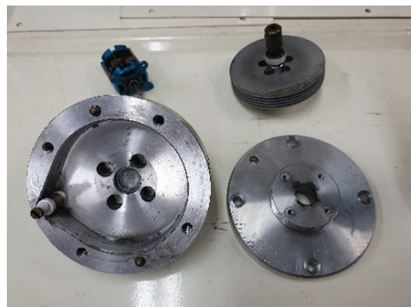
Fig. 5 Tesla turbine open view
