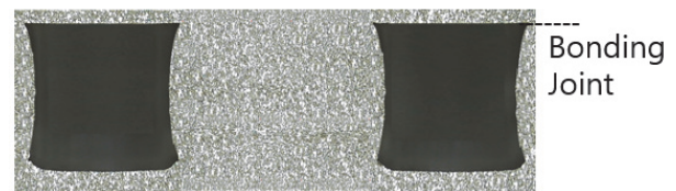
Fig. 2 Multi-channel cross-section after bonding
