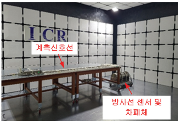
Fig. 9 Electro Magnetic testing chamber
